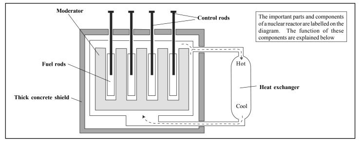
**Moderator** - In naturally occurring uranium only about 1 atom in 140 is a uranium 235  $\binom{235}{92}$ U) isotope. The rest of the atoms are uranium 238  $\binom{238}{92}$ U).
